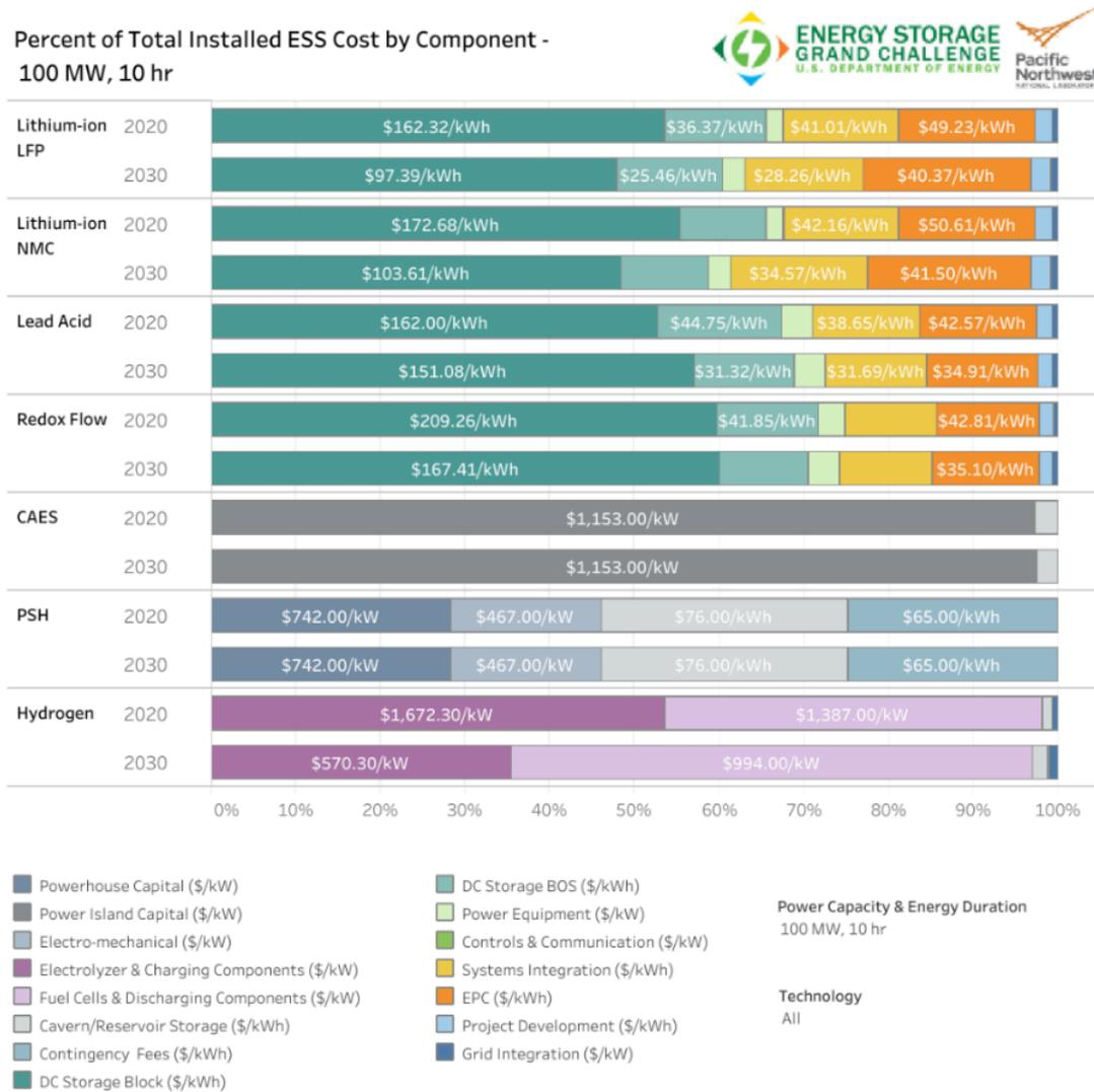
Figure 59: The percentage of total installed electricity storage costs by cost component for each technology.<sup>163</sup> This illustrates the breakdown of cost components within each storage technology and how each contributes to the total installed cost.
