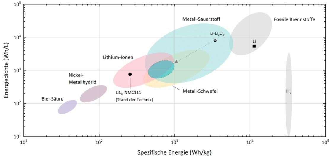
Figure 47: Energy density of different battery types.
