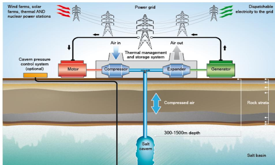
Figure 53: Compressed air storage system.
