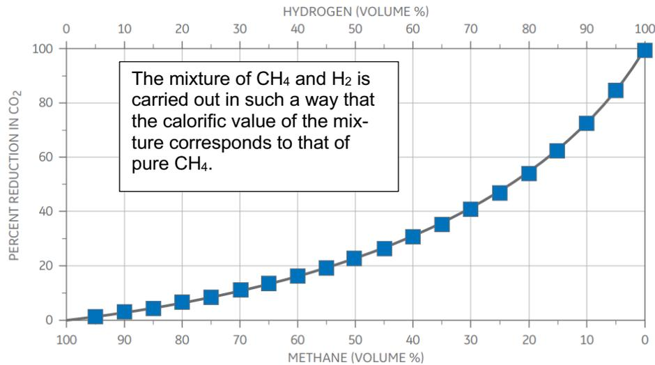
Figure 51: Ratio of carbon dioxide emissions and volume flow for a fuel mixture of methane and hydrogen for the same calorific value
