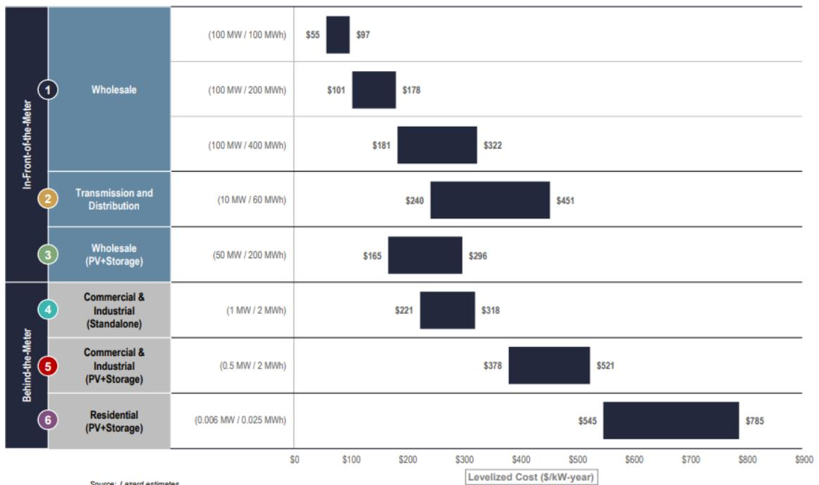
Figure 54: Electricity storage cost (LCOS) of lithium batteries and redox flow batteries for different applications and based on storage capacity.
