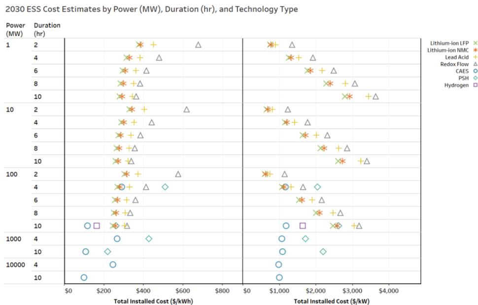
Figure 60: Installation costs (USD/kW) and storage costs by storage capacity (USD/kWh) of various types of electricity storage.<sup>166</sup>
