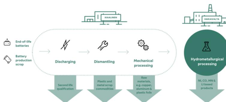
Figure 64: The lithium-ion battery recycling process.
