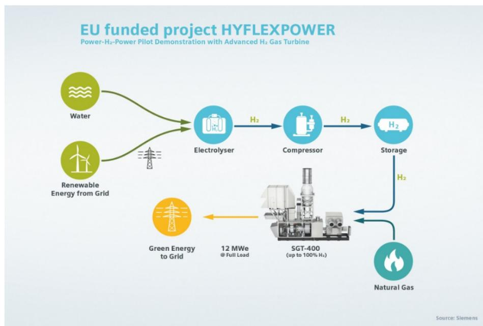
Figure 50: Power-to-Hydrogen-to-Power Model.
