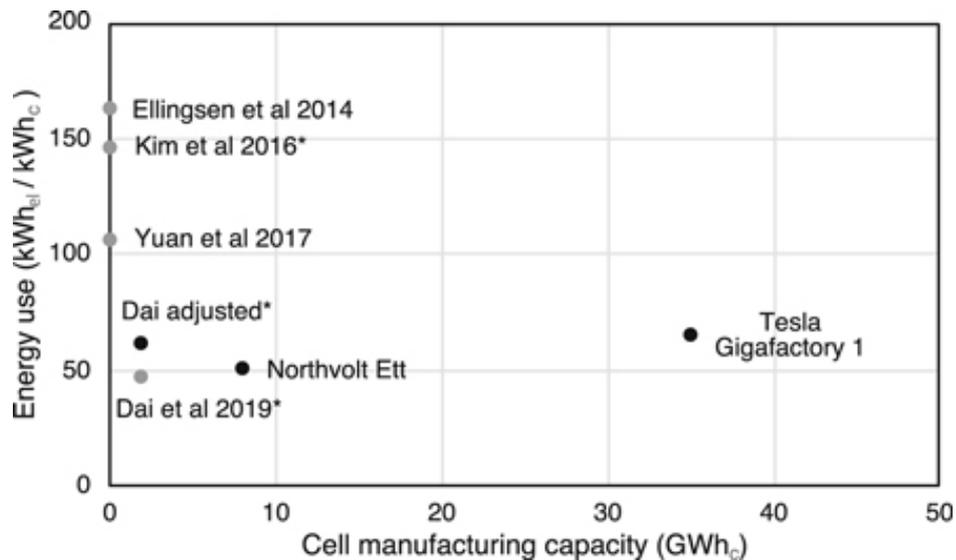
Figure 63: Electricity demand per kWh of lithium-ion electricity storage capacity.
