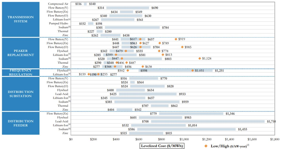
Figure 56: Electricity storage costs (LCOS) of CAES, pumped storage power plant for various purposes in the electricity grid (ordered by storage capacity).
