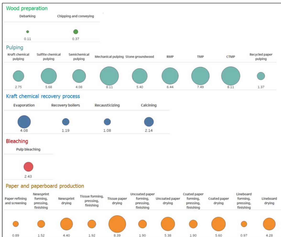
Figure 44 : Average energy consumption in GJ/tonne for pulp and paper manufacturing processes.
